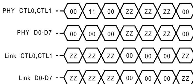
2. To cancel after asserting Hold, assert Idle between two cycles; it switches to high impedance. This method cancels the packet transmission connection (concatenated) after Grant is received. The μPD72852 cancels with the next Idle cycle of Hold. To prevent CTL from switching to high impedance, assert a second Idle cycle.
