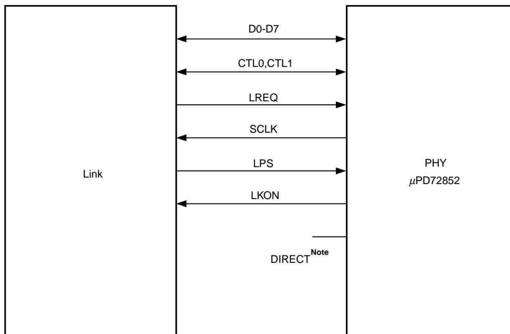
**Note** Clamping to V<sub>DD</sub> provides direct connection to Link.
