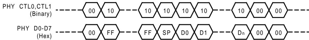
The packet transfer rate of the serial bus depends on the topology of the bus. The μPD72852 checks if the node can receive at the faster transfer rate. At this time, DATA\_PREFIX → DATA\_END is transmitted to the μPD72852. After DATA\_PREFIX is transmitted to the Link, Receive from the serial bus is completed, asserting Idle.
