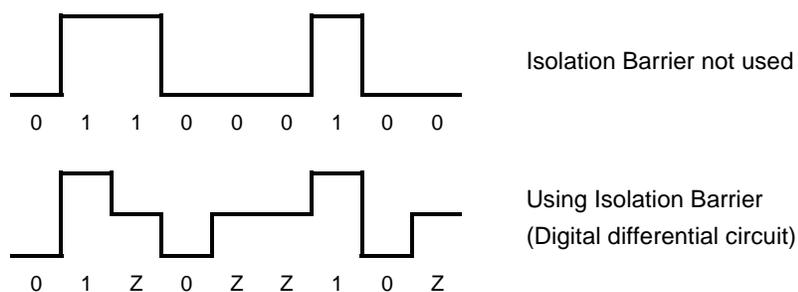
★ Figure 3-3. Isolation Barrier Circuits
