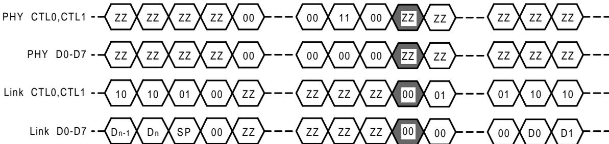
**Note** In case of packet transmission after Grant, before actual transmission, Hold does not need to be asserted.
