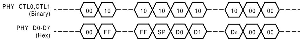
The packet transfer rate of the serial bus depends on the topology of the bus. The μPD72850A checks if the node can receive at the faster transfer rate. At this time, DATA\_PREFIX → DATA\_END is transmitted to the μPD72850A. After DATA\_PREFIX is transmitted to the Link, Receive from the serial bus is completed, asserting Idle.
