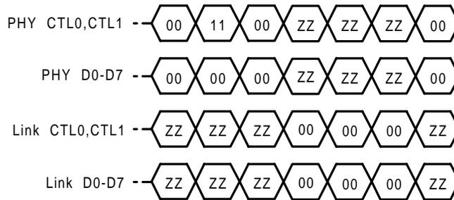
2. To cancel after asserting Hold, assert Idle between two cycles; it switches to high impedance. This method cancels the packet transmission connection (concatenated) after Grant is received. The μPD72850A cancels with the next Idle cycle of Hold. To prevent CTL from switching to high impedance, assert a second Idle cycle.
