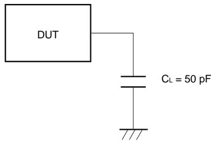
**Caution** If the load capacitance exceeds 50 pF due to the configuration of the circuit, keep the load capacitance of this device to within 50 pF by inserting a buffer or by some other means.
