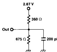
Loading Conditions: I<sub>OL</sub> = 12 mA, I<sub>OH</sub> = 4 mA, C<sub>L</sub> = 200 pF
