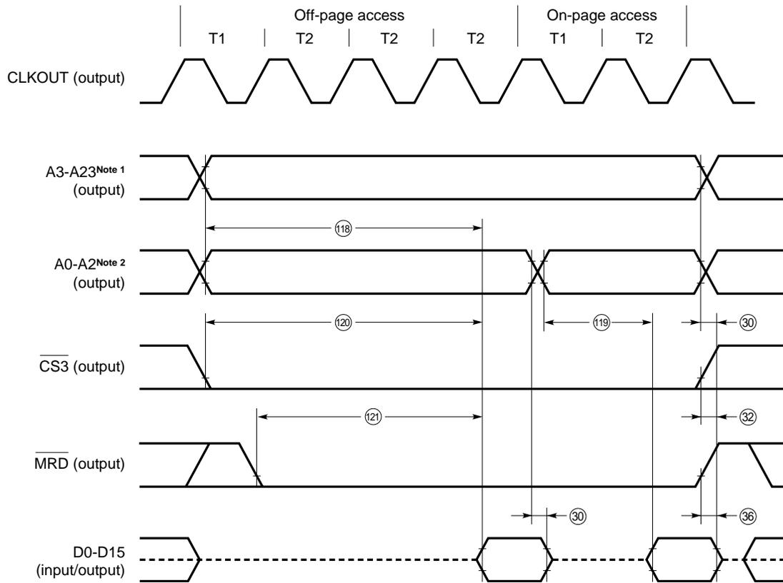
**Notes 1.** The address pins to be used vary with the settings of bits MA5 to MA3 of the page-ROM configuration register (PRC).
