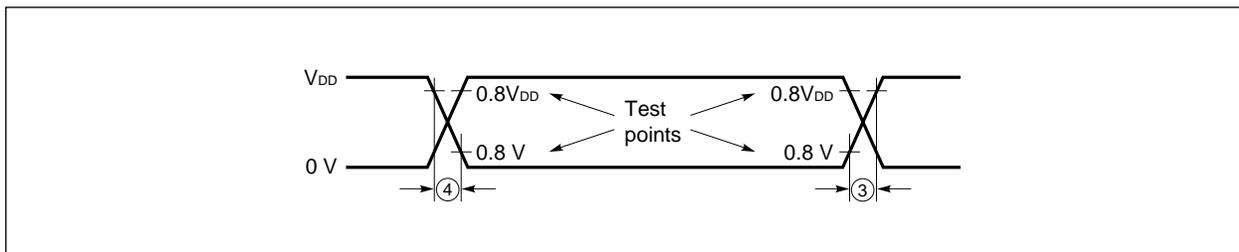
**AC Test Output Waveform**
