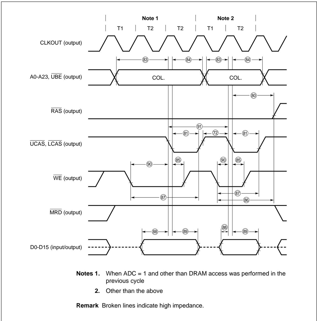
(6) DRAM access timing (when a control circuit is configured using a gate array or other devices)
