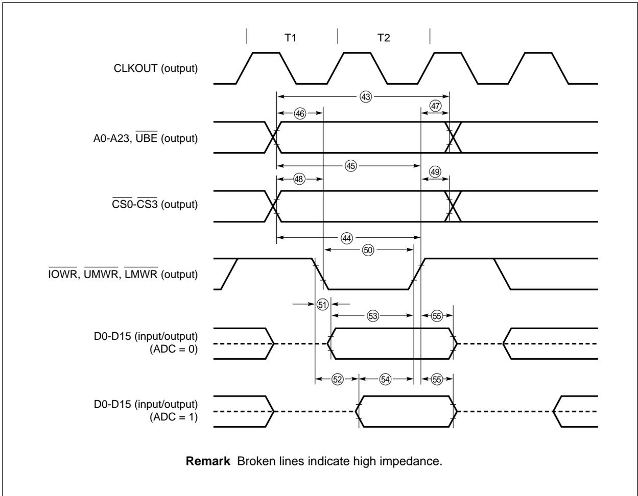
(5) DRAM access timing (when DRAM is directly connected)
