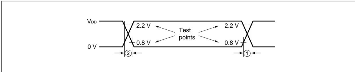
**AC Test Input Waveform ( $\overline{\text{RESET}}$ ,  $\overline{\text{NMI}}$ , and  $\overline{\text{INTPn}}$ )**
