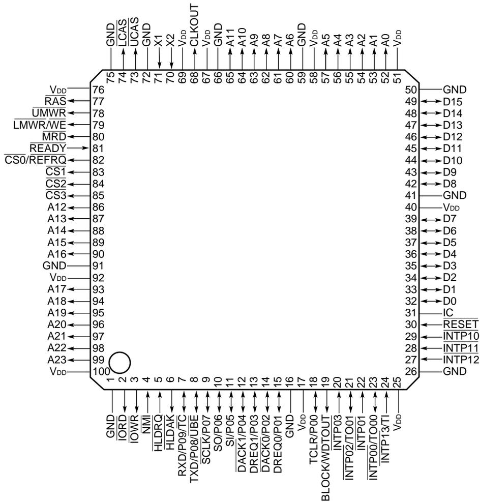
Caution Connect the IC pin to GND through a resistor.
