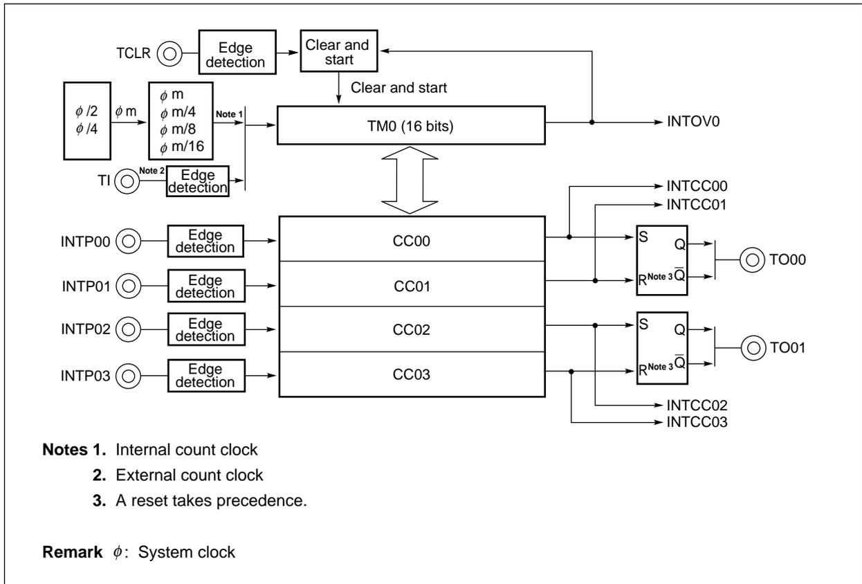
Figure 9-2. Timer 1 (16-Bit Interval Timer)
