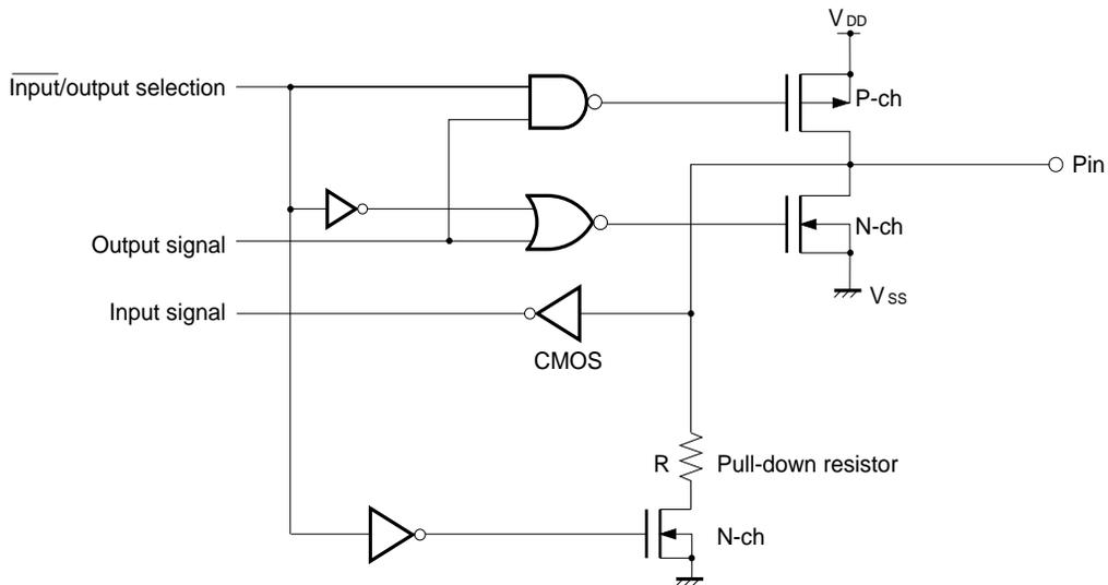
When K<sub>I/O</sub> is set to the input mode, pull-down resistor R is turned on.
