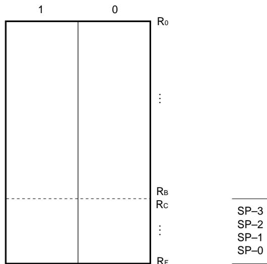
**Caution** Avoid using the RAM areas R<sub>D</sub>, R<sub>E</sub>, and R<sub>F</sub> in a CALL routine as much as possible because these areas are also used as stack memory areas (to prevent program hang-up in case the value of the SP is destroyed due to some reason such as noise).
