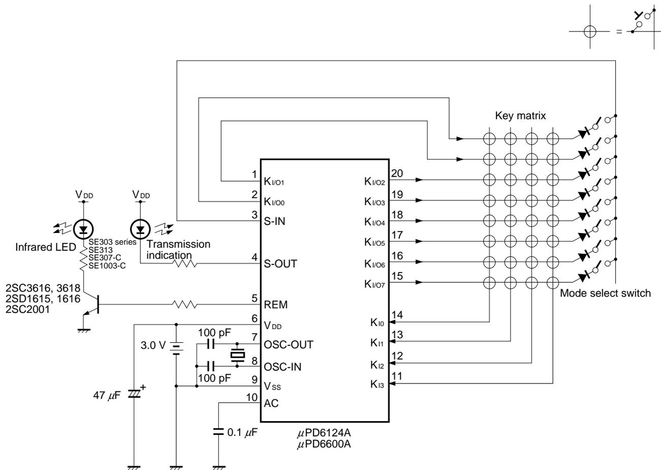
**Caution** The ceramic resonator start up capacitor value must be determined, by taking the voltage level and the oscillation start up characteristics for the ceramic resonator into consideration.
