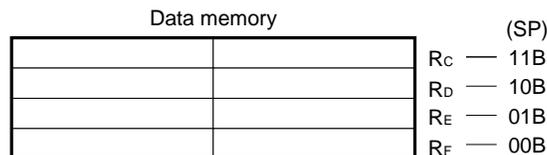
If the stack pointer overflows or underflows, it is determined that the CPU overflows, and the PC internal reset signal will be generated.
