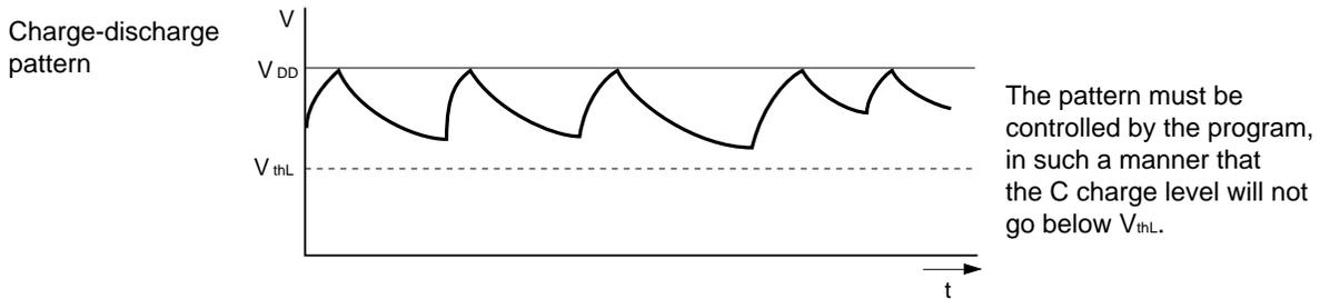
**Caution** When the watchdog timer function is not used, switch to charging mode by executing a NOP instruction immediately before a HALT instruction at the beginning of the program. (Be sure to connect the capacitor.)
