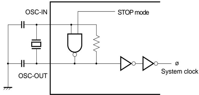
In the STOP mode (oscillation stop HALT instruction), the oscillator in the system clock generator stops its operation, and the system clock ø is stopped.
