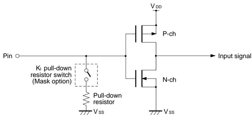
When the pull-down resistor switch is turned on (set 1) by the mask option, pull-down resistor R is turned on.
