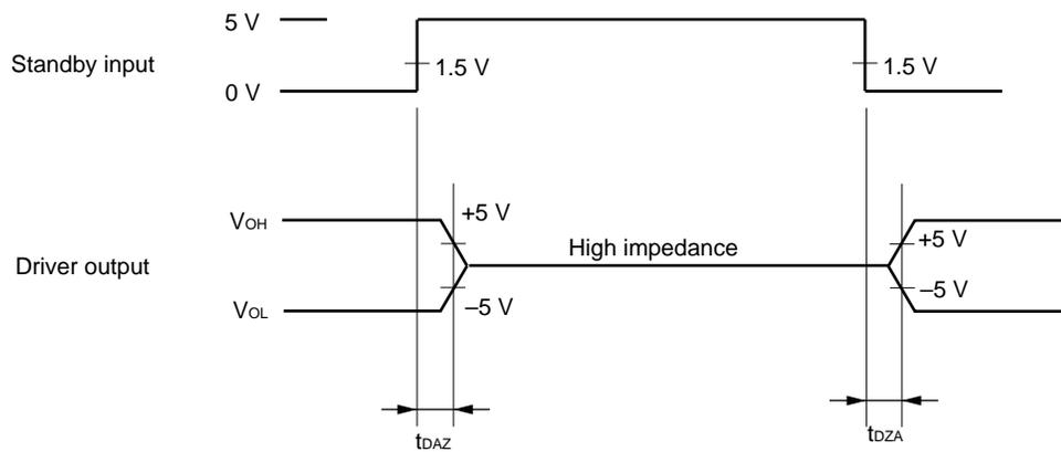
Do not perform communication within the standby output transition time t<sub>DZA</sub> on power application or on releasing the standby mode.
