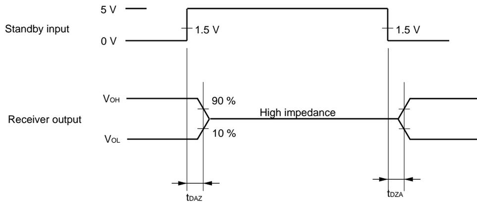
The receiver output is undefined during the standby output transition time  $t_{DZA}$ . Do not perform communication in the standby output transition time  $t_{DZA}$  on power application or on releasing the standby mode.
