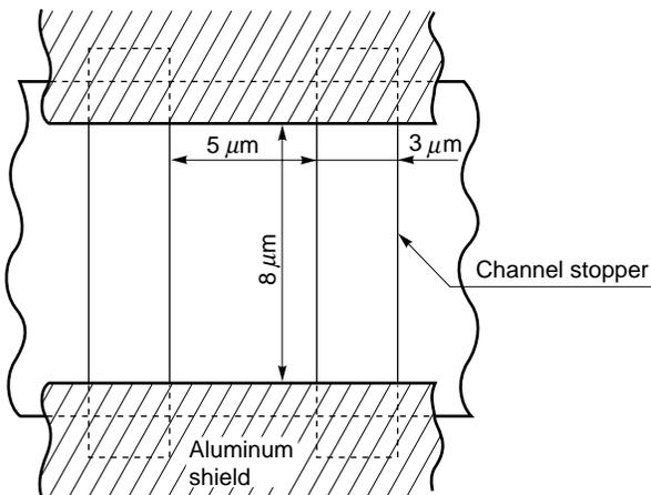
**PHOTOCELL ARRAY STRUCTURE DIAGRAM (Line spacing)**
