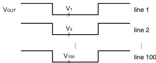
This is measured by the DC level sampling of only the signal level, not by CDS (Correlated Double Sampling).
