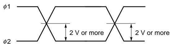
**Remark** Adjust cross points of  $\phi_1$  and  $\phi_2$  with input resistance of each pin.
