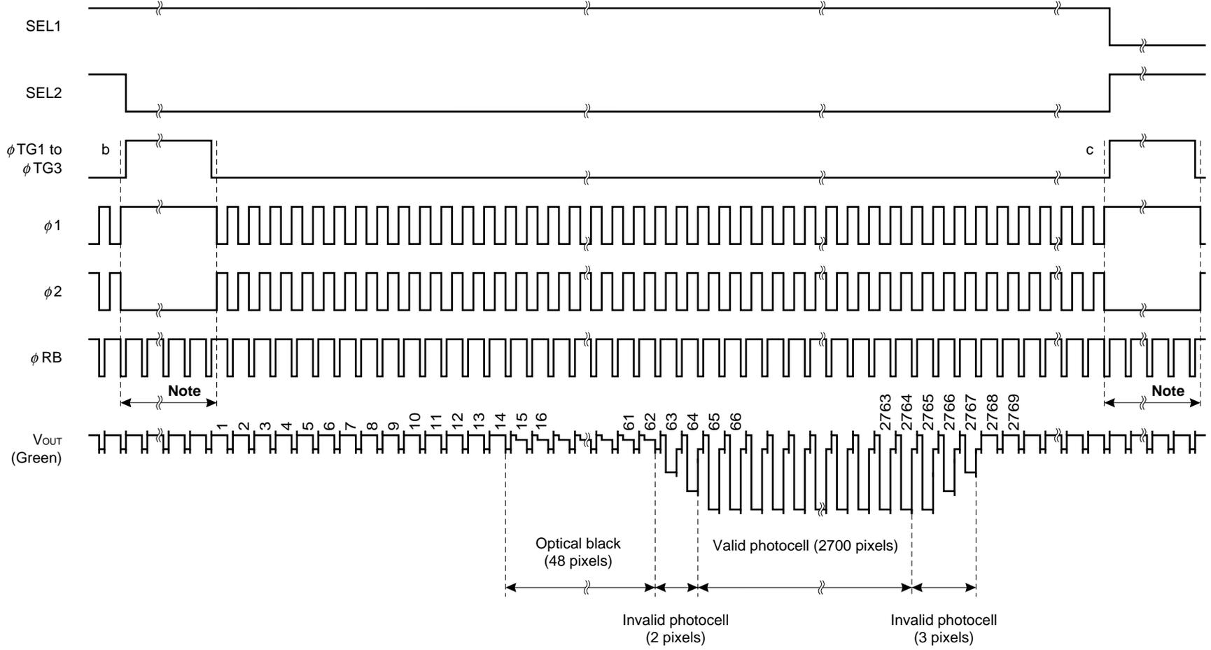
**Note** Input the  $\phi$ RB pluse continuously during this period, too.
