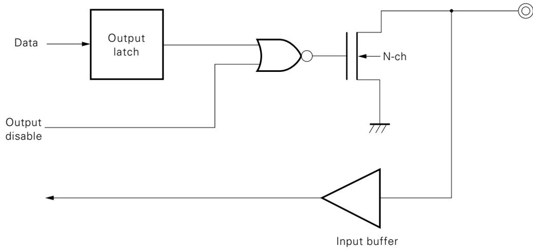
(3) P1A<sub>0</sub>-P1A<sub>3</sub>, P1B<sub>0</sub>-P1B<sub>3</sub>/TM2OUT
