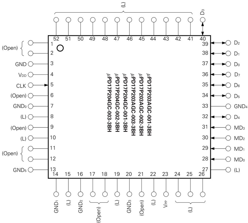
**Caution** Those enclosed in parentheses indicate the processing of the pins not used in PROM programming mode.
