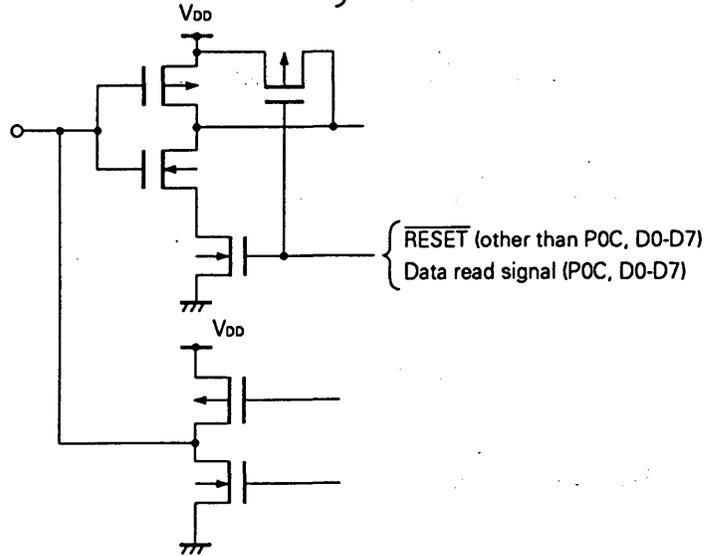
\* :The  $\overline{\text{RESET}}$  signal is not supplied to P0C and D0-D7.
