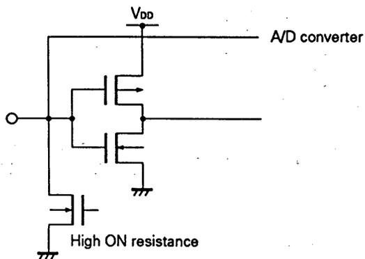
1.3.6 P1D (P1D<sub>1</sub>/ADC<sub>1</sub>, P1D<sub>0</sub>/ADC<sub>0</sub>) (Input)
