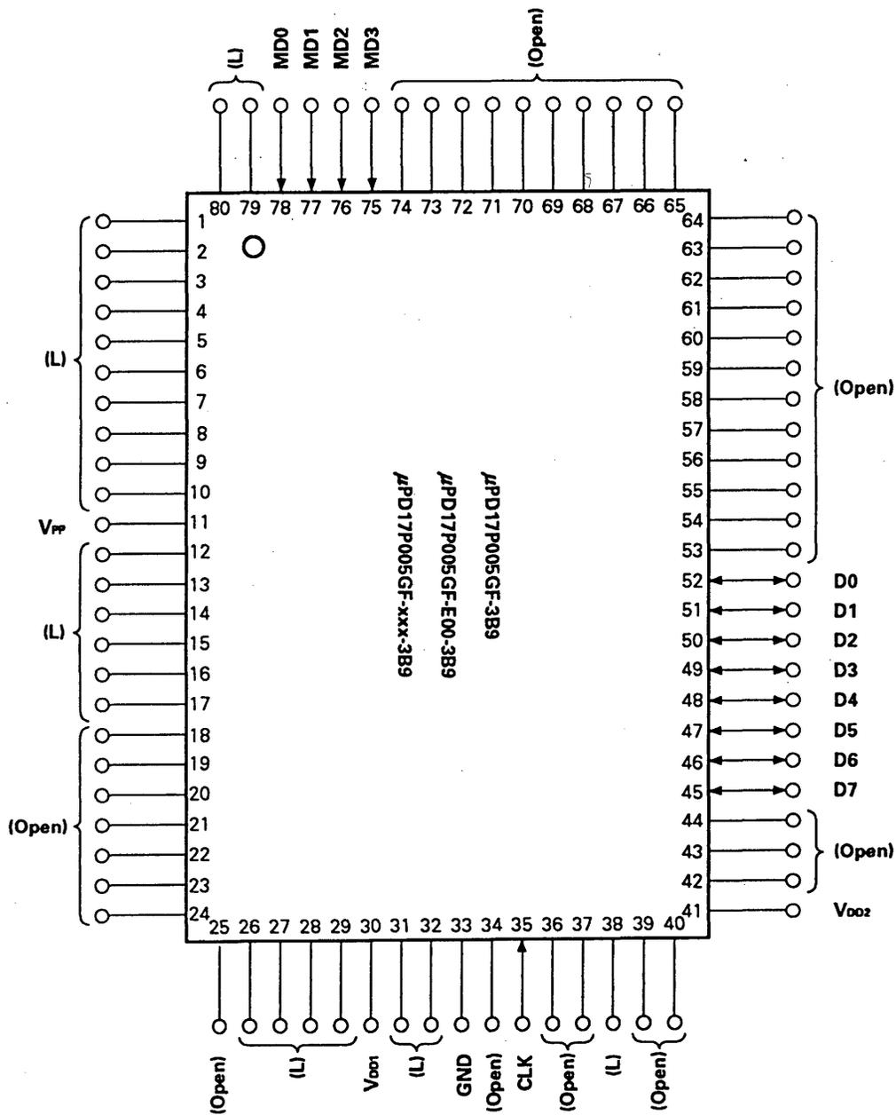
**Note:** ( ) indicates the processing of the pins not used in the PROM programming mode.
