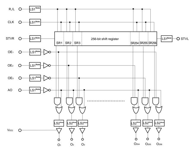
Note LS1: shifts CMOS level and internal level, LS2: shifts interval level and output level (VDD2-VEE2).
