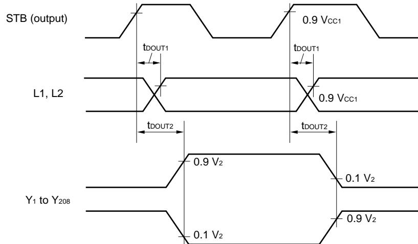
**AC Characteristics 2 Drawing Access Timing**
