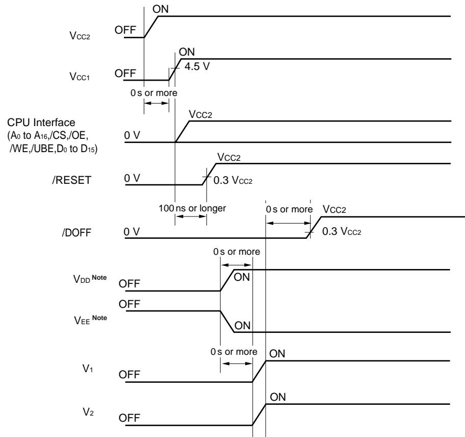
**Note**  $V_{DD}$  and  $V_{EE}$  do not have to be turned ON at the same time.
