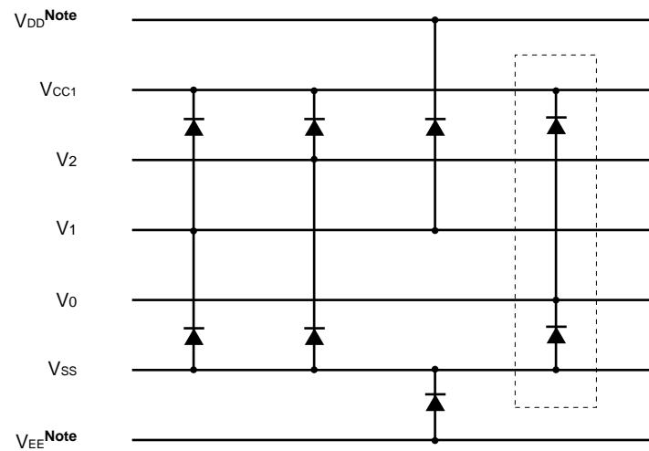
[Dashed Box] Diodes enclosed in a dotted line in the above figure must be connected when  $V_0$  is other than 0 V (GND).
