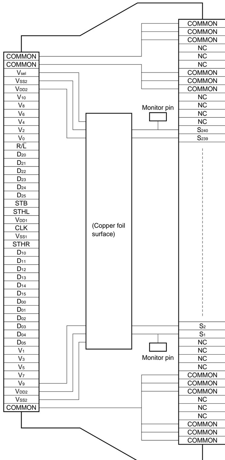
V<sub>sel</sub> pin is internally pulled up.
