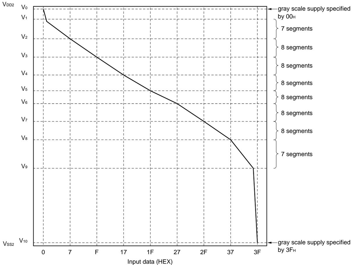
Relation between Input Data and Output Voltage
