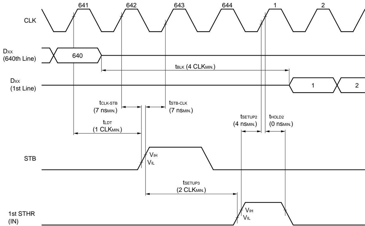
9. DATA INPUT TIMING IN CASCADE CONNECTION
