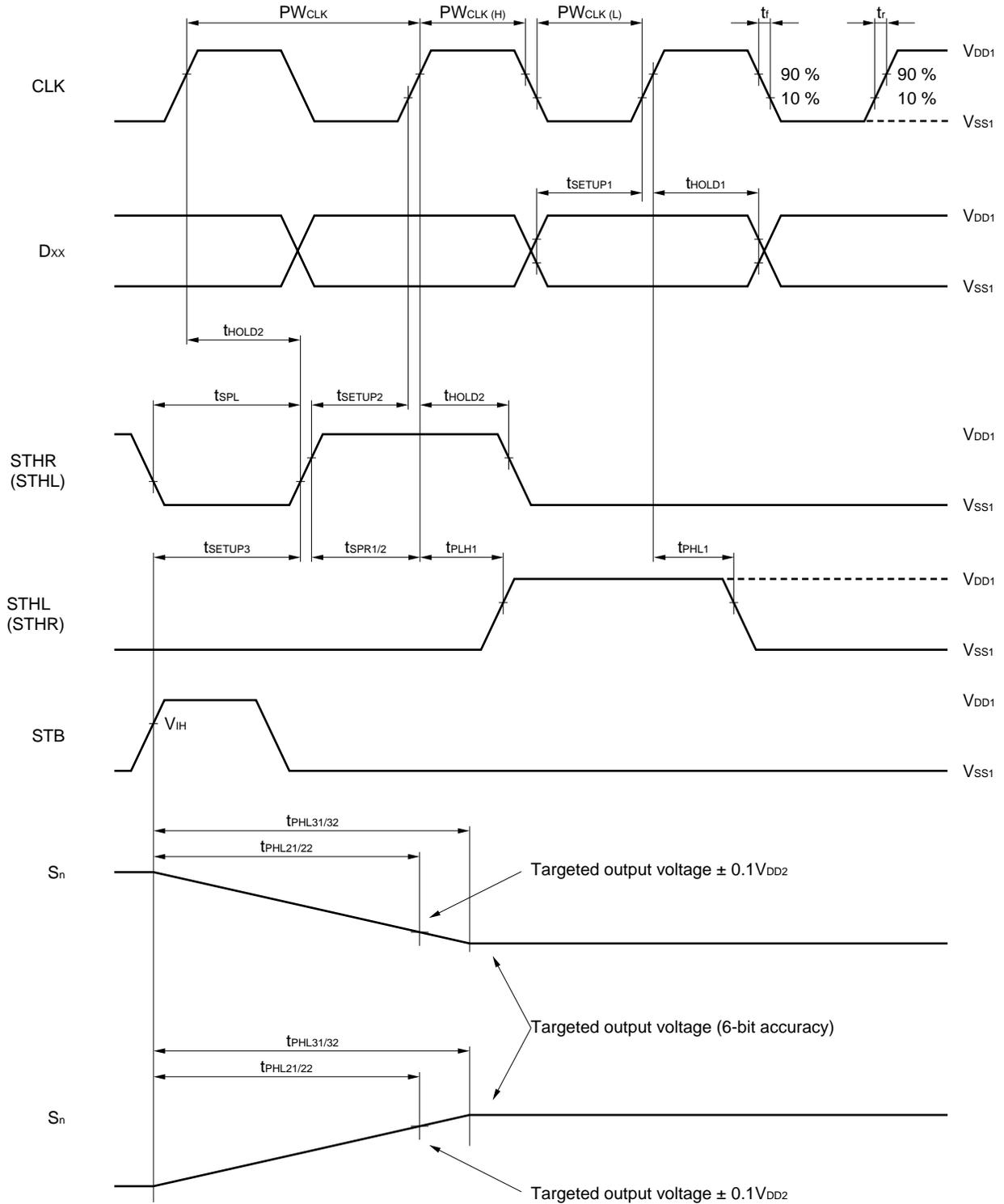
Switching Characteristic Waveform
