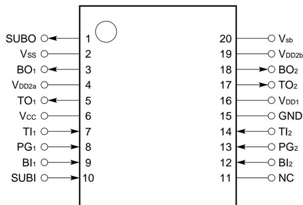
**Remark** The μPD16510 is pin-compatible with the μPD16506 (CCD driver). However, the VOD shutter drive pulse input polarity switching pin (SSP) of the μPD16506 corresponds to the GND pin in the μPD16510 (pin 15).
