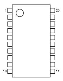
1. UHF OSC Collector (Tr. 1) 2. UHF OSC Base (Tr. 2) 3. UHF OSC Base (Tr. 1) 4. UHF OSC Collector (Tr. 2) 5. UB 6. OSC OUTPUT 7. GND 8. VHF OSC Base (Tr. 1) 9. VHF OSC Base (Tr. 2) 10. VHF OSC Collector (Tr. 1) 11. REG 12. IF OUTPUT 13. Vcc 14. MIX OUTPUT 15. MIX OUTPUT 16. VHF RF INPUT 17. VHF RF INPUT 18. GND 19. UHF RF INPUT
