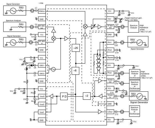
NOTE: Spectrum Analyzer to measure frequency. Oscilloscope to measure voltage swing.
