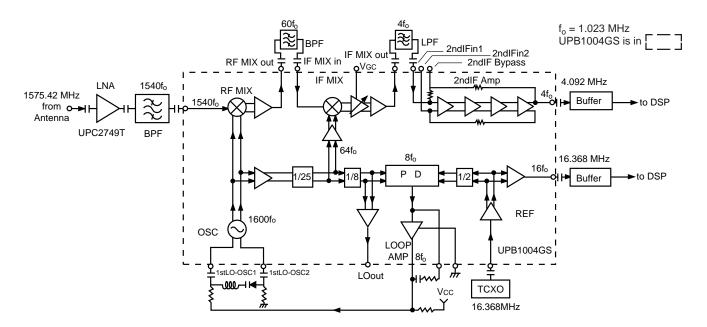
Note: This diagram schematically shows only the UPB1004's internal functions on the system. This diagram does not represent the actual application circuit.
