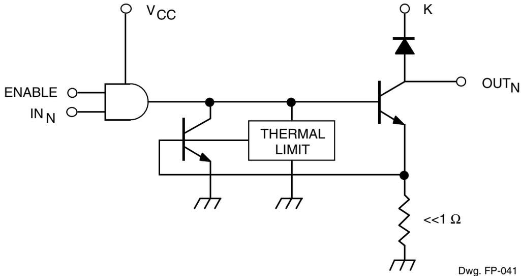
NOTE: These devices do not include an absolute thermal shutdown. Package power dissipation under fault conditions (2.4 W in the faulted channel) must therefore be evaluated at maximum operating temperature.
