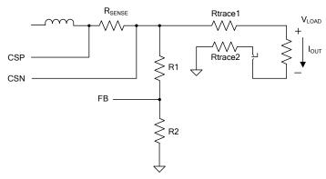
$I_{OUT} \times RSENSE \times 20\mu \times R1 = I_{OUT} \times Rtrace$
