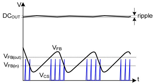
Fig.8 DC Output, V<sub>FB</sub>, V<sub>CS</sub> Timing
