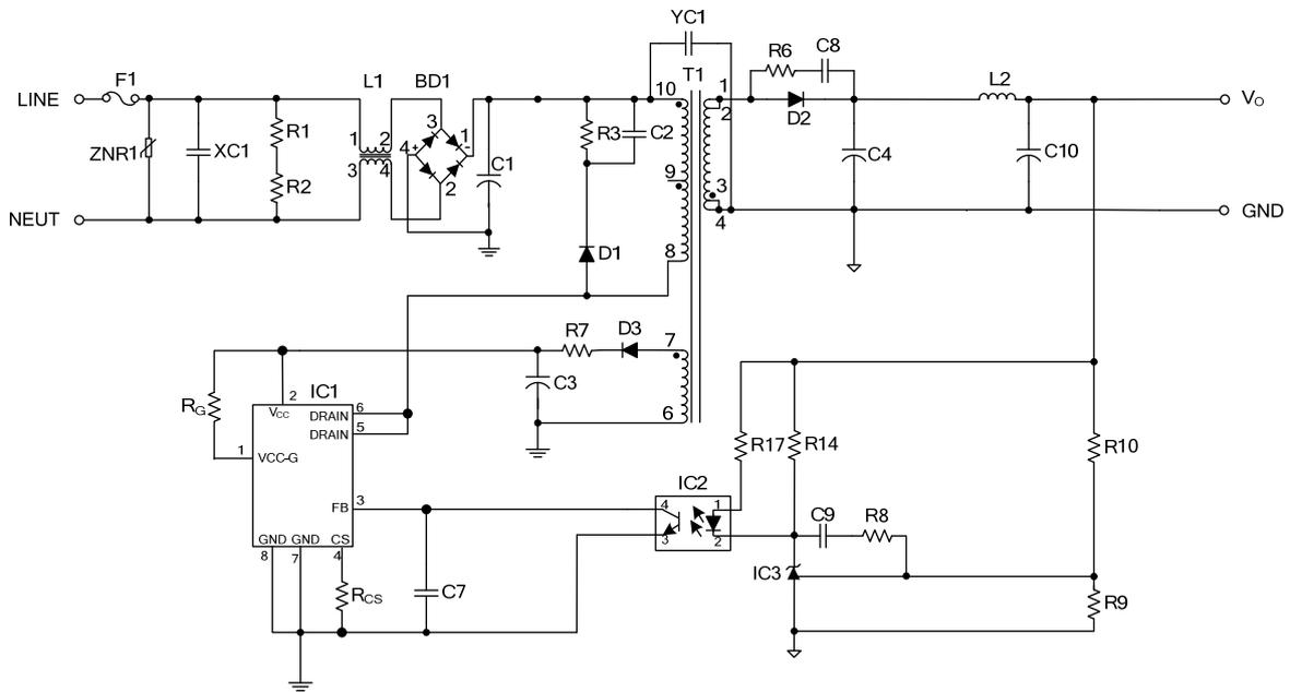
Fig.8 UTC UCS16505S Typical Application Circuit
