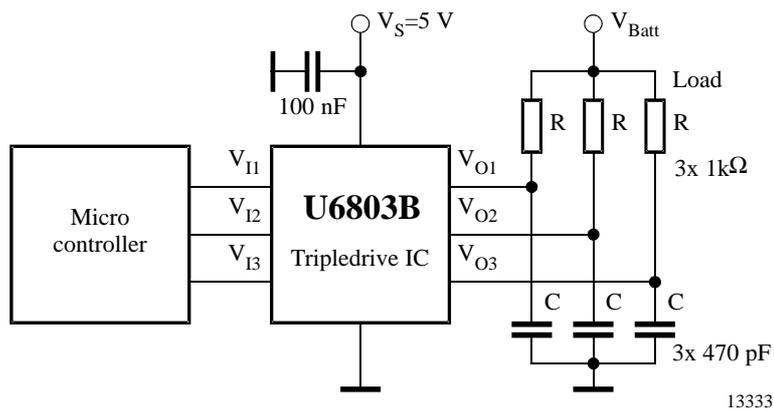
Figure 3. Application schematic
