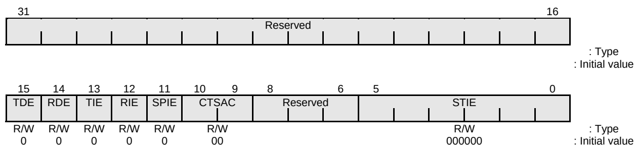
Figure 19-7 DMA/Interrupt Control Register
