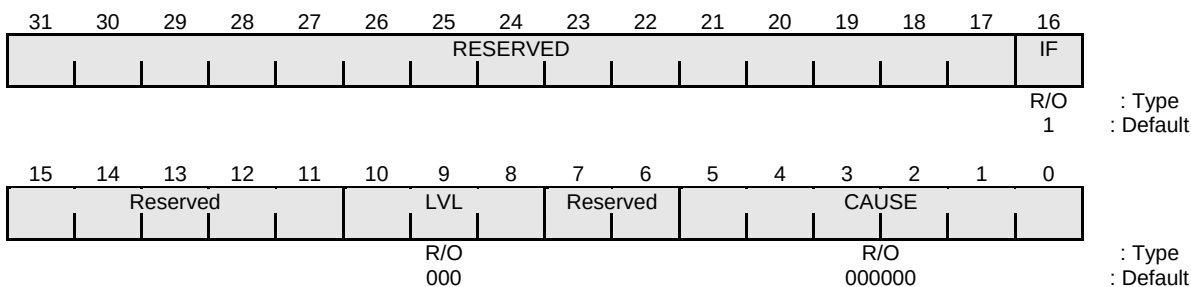
Figure 8-15 Interrupt Current Status Register
