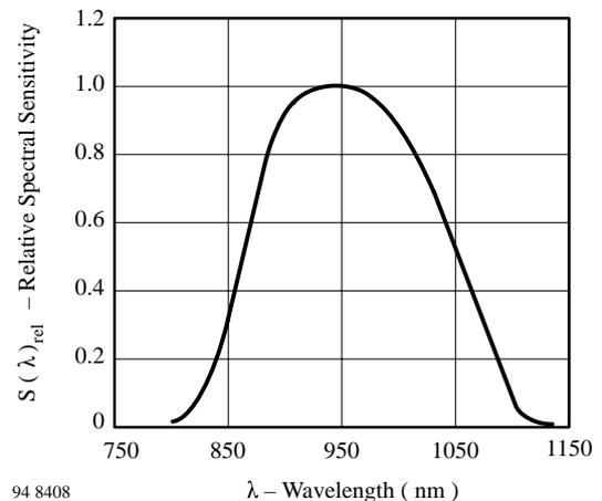
Figure 12. Relative Spectral Sensitivity vs. Wavelength
