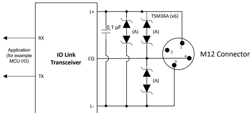
A. Diagram shows two TSM36A unidirectional devices stacked in series with the anodes tied back-to-back to protect between the respective signals.
