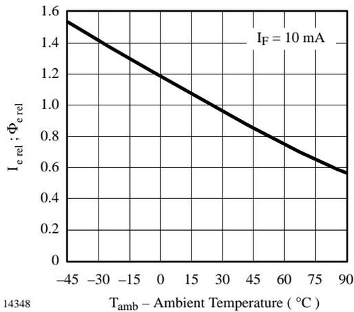
Figure 7. Relative Radiant Intensity vs. Ambient Temperature
