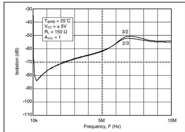
**INPUT/OUTPUT ISOLATION IN STANDBY MODE (SO16 PACKAGE)**
