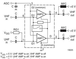
GG = 0 V: UHF AMP is off; VHF AMP is or (0 = shorted to Ground or open)
