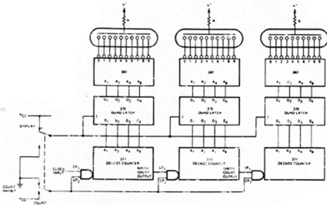
This circuit counts, stores, and displays the count. When the switch is in the count position, the decade counters count clock pulses and the indicator tubes display the count being held in the quad latches. When the switch is moved to the display/count inhibit position the counters stop counting; the number at which they were stopped is transferred to storage and the display tubes change to the new number. If the switch is then returned to its original position the circuit will resume counting.
