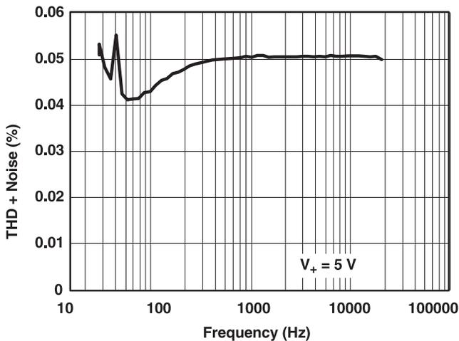
Figure 11. Total Harmonic Distortion vs Frequency (V<sub>+</sub> = 5 V)
