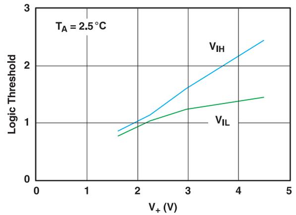
Figure 8. Logic-Level Threshold vs V<sub>+</sub>
