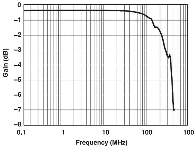
Figure 9. Frequency Response (V<sub>+</sub> = 3 V)
