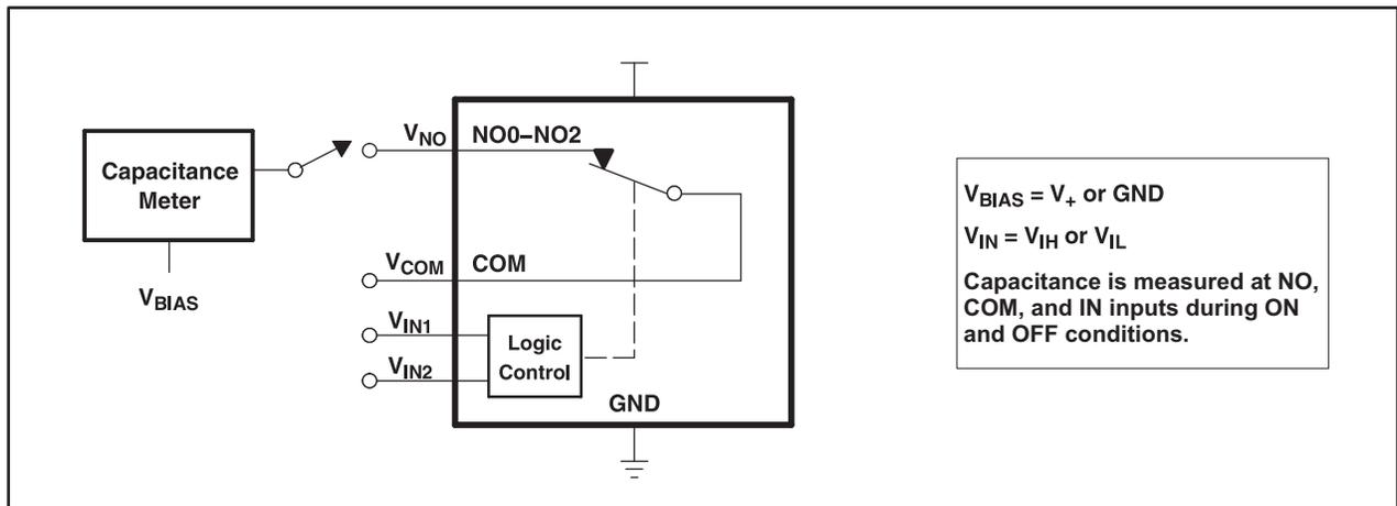
Figure 15. Capacitance ( $C_I$ ,  $C_{COM(ON)}$ ,  $C_{NO(OFF)}$ ,  $C_{COM(OFF)}$ ,  $C_{NO(ON)}$ )
