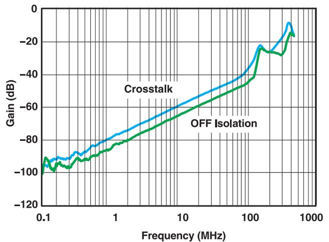
Figure 10. OFF Isolation and Crosstalk vs Frequency (V<sub>+</sub> = 3 V)
