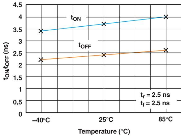
Figure 7. t<sub>ON</sub> and t<sub>OFF</sub> vs Temperature (V<sub>+</sub> = 5 V)
