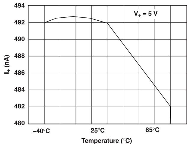
Figure 12. Power-Supply Current vs Temperature (V<sub>+</sub> = 5 V)
