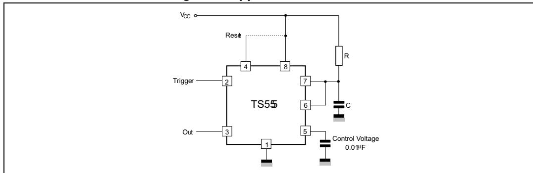
The circuit triggers on a negative-going input signal when the level reaches  $1/3 V_{CC}$ . Once triggered, the circuit remains in this state until the set time has elapsed, even if it is triggered again during this interval. The duration of the output HIGH state is given by  $t = 1.1 R \times C$ .
