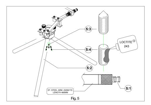
• Remove the grease from the thread (5:1) of the arms (5:2) with trichlorethylene (care must be taken when using any substance or chemical that can be harmful, refer to the manufacturer's information and/or a Health & Safety "Risk Assessment") and apply some Loctite® 243 (blue) or an equivalent industrial bonding adhesive on the thread.
