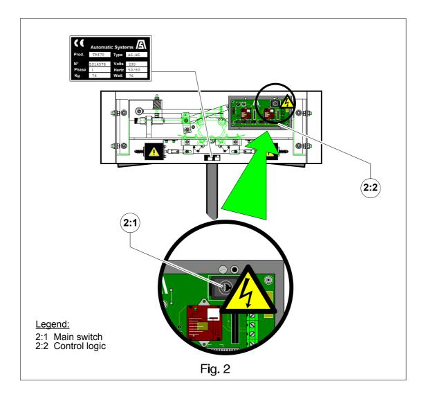
• As soon as you open the housing, put off the main switch (2:1) on the electrical control logic (2:2), located under the hood.
