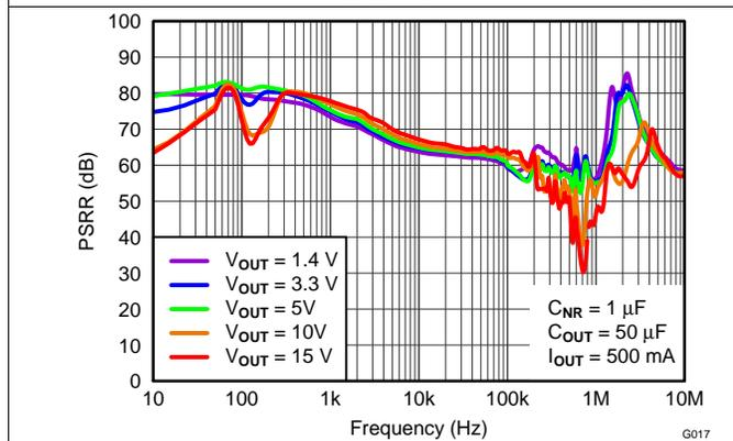
Figure 17. Power-Supply Rejection Ratio vs Output Voltage
