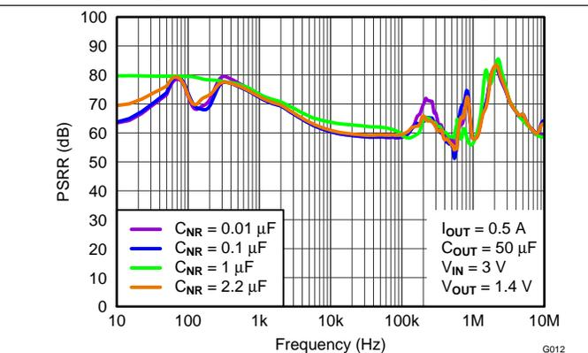
Figure 12. Power-Supply Rejection Ratio vs  $C_{\text{NR}}$
