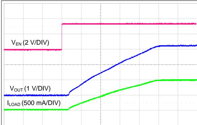
Figure 25. Startup with EN Pin rising (10 ms/DIV)
