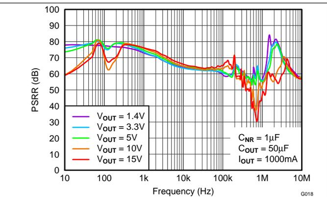
Figure 18. Power-Supply Rejection Ratio vs Output Voltage
