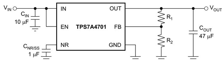
**Figure 23. Adjustable Operation for Maximum AC Performance**
