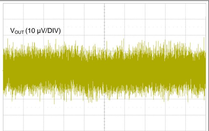
Figure 26. Output Noise Voltage, 10 Hz to 100 kHz (10 ms/DIV)
