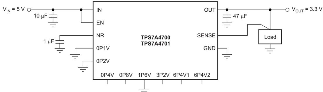
**Figure 24. Typical Application,  $V_{OUT} = 3.3\text{ V}$**
