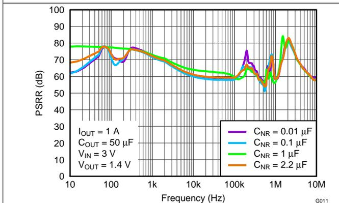
Figure 11. Power-Supply Rejection Ratio vs  $C_{\text{NR}}$
