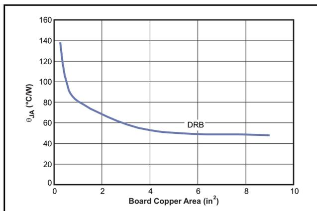
Note:  $\theta_{JA}$  value at board size of 9 in<sup>2</sup> (that is, 3 in × 3 in) is a JEDEC standard.
