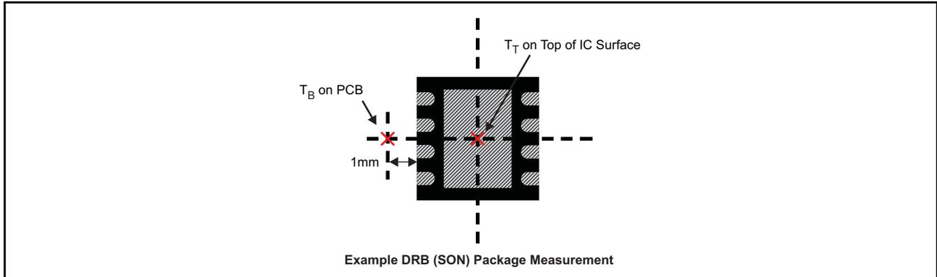
Figure 27. Measuring Point for T<sub>T</sub> and T<sub>B</sub>
