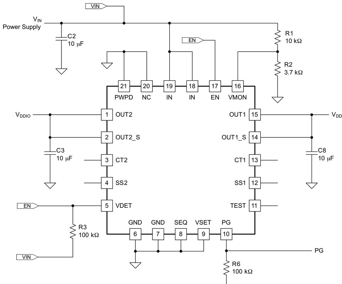
**Figure 25. Configuration for F280x, F281x, F223x and F2833x Controllers
