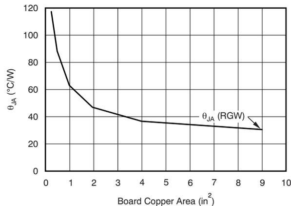
NOTE:  $\theta_{JA}$  value at a board size of 9-in<sup>2</sup> (that is, 3-in × 3-in) is a JEDEC standard.
