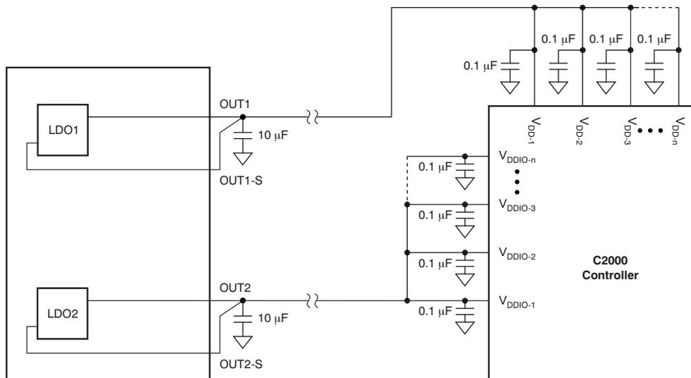
**Figure 27. Output Capacitors Placement and Sense Pins**
