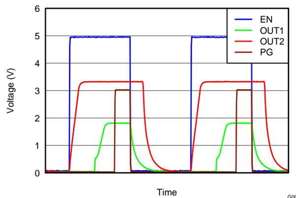
**Figure 31. Power Sequence with SEQ = H**
