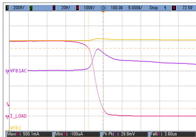
Figure 7-2. VDD1 Falling Load Transient Response
