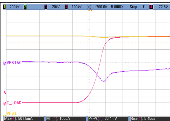
Figure 7-3. VDD1 Rising Load Transient Response
