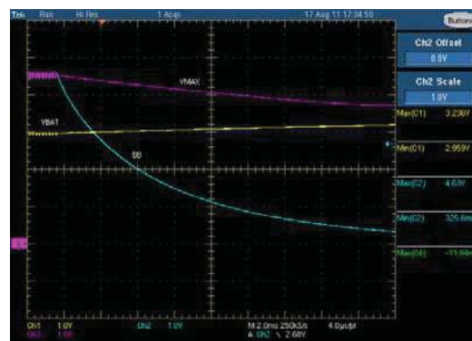
Figure 50. VMAX waveform. Falling BB output. Switch configured for VMAX = MAX(VBAT, VBBout)-diode when BB output is disabled. Note: VMAX is not loaded.
