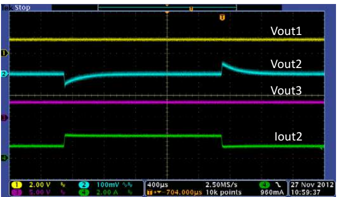
Figure 23. Transient Response Buck2 @ 1.8V, 1-2A Step, C_o = 47\mu\text{F}
