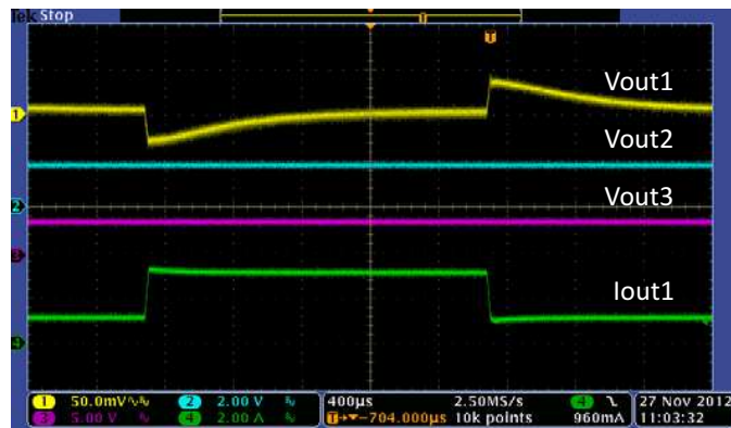
Figure 22. Transient Response Buck1 @ 1.2V, 1-3A Step, C_o = 68\mu\text{F}
