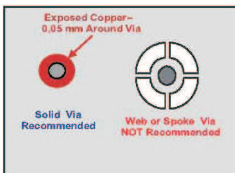
Figure 27. Thermal Via Connection at the Bottom Layer
