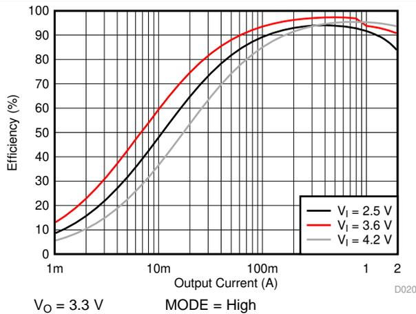
Figure 18. Efficiency versus Output Current (PWM Only)
