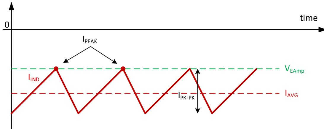
**Figure 8. Peak-Current Operation, Reverse Current**
