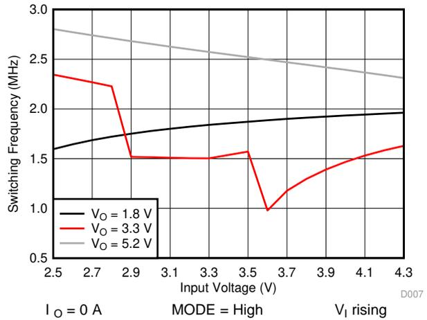
Figure 15. Typical Inductor Switching Frequency versus Input Voltage
