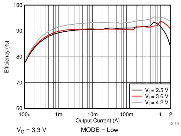
Figure 17. Efficiency versus Output Current (PFM/PWM)
