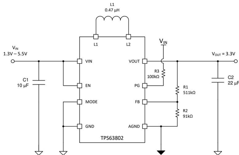
Figure 13. 3.3 V<sub>OUT</sub> Typical Application
