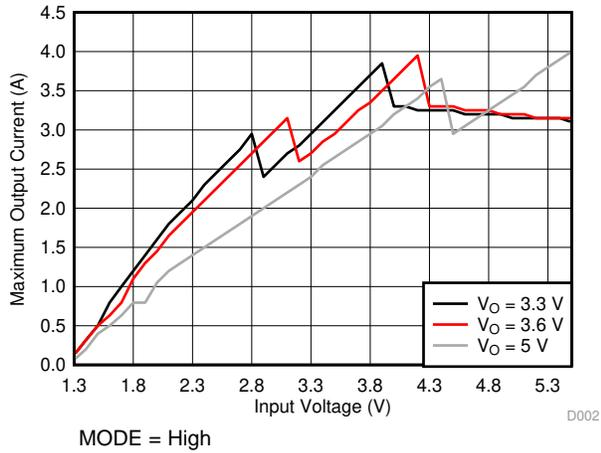
Figure 14. Typical Output Current Capability versus Input Voltage
