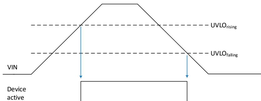
Figure 5. Rising and Falling Undervoltage Lockout Behavior
