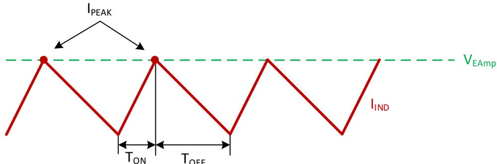
**Figure 9. Peak-Current Boost Operation**
