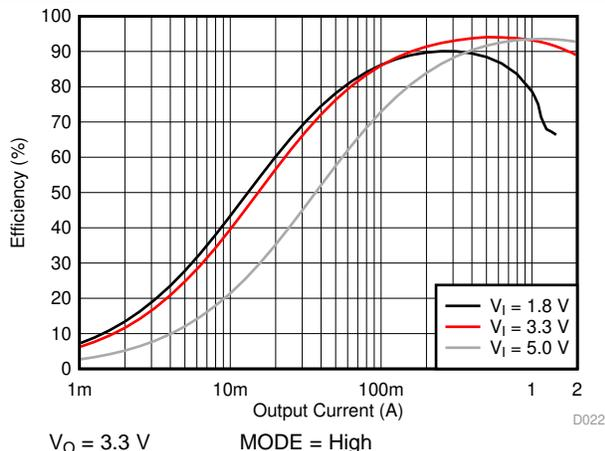
Figure 20. Efficiency versus Input Voltage (PWM Only)
