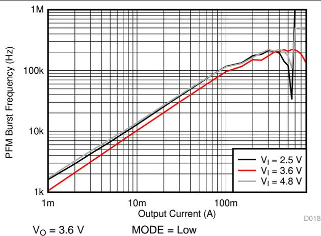
Figure 16. Typical Inductor Burst Frequency versus Output Current
