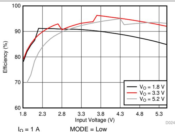
Figure 22. Efficiency versus Input Voltage (PWM Only)
