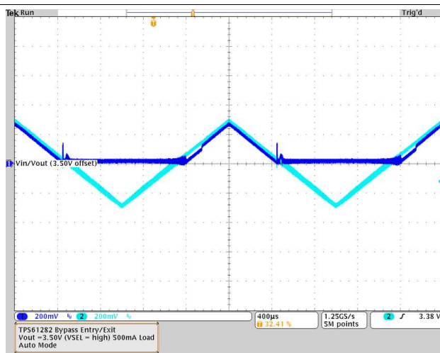
Figure 59. Boost to Pass-Through Mode Exit / Entry
