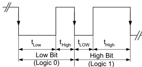
**Figure 13. EasyScale — Bit Coding**
