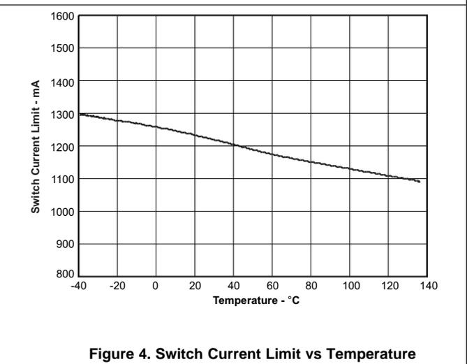
**Figure 4. Switch Current Limit vs Temperature**
