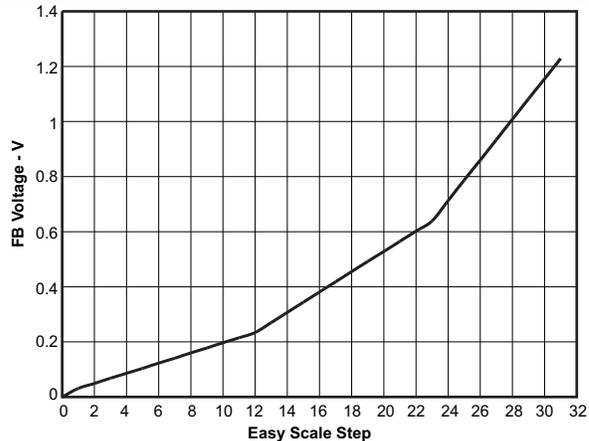
Figure 6. FB Voltage vs EasyScale Step
