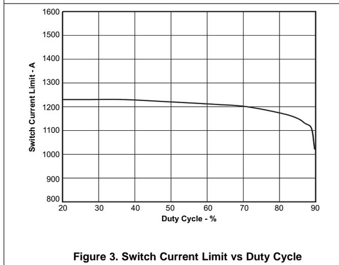
**Figure 3. Switch Current Limit vs Duty Cycle**
