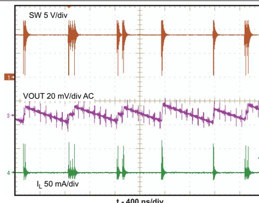
Figure 10. Skip-Cycle Switching
