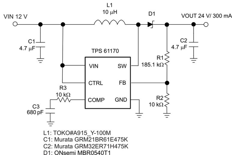
**Figure 15. 12-V to 24-V DC-DC Power Conversion**
