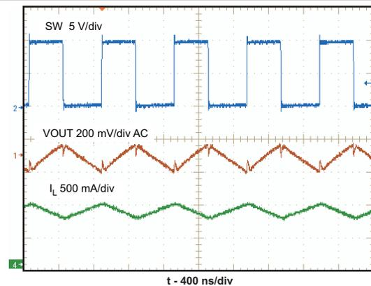
Figure 8. Switching Waveform
