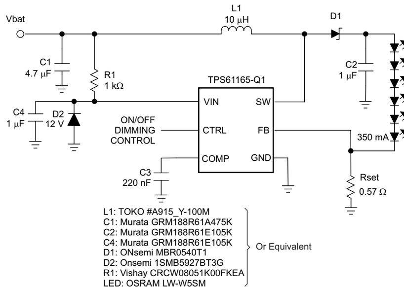
Figure 15. Drive Six High-Brightness LEDs
