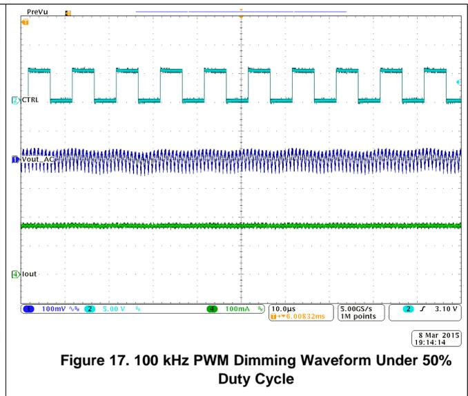
Figure 17. 100 kHz PWM Dimming Waveform Under 50% Duty Cycle
