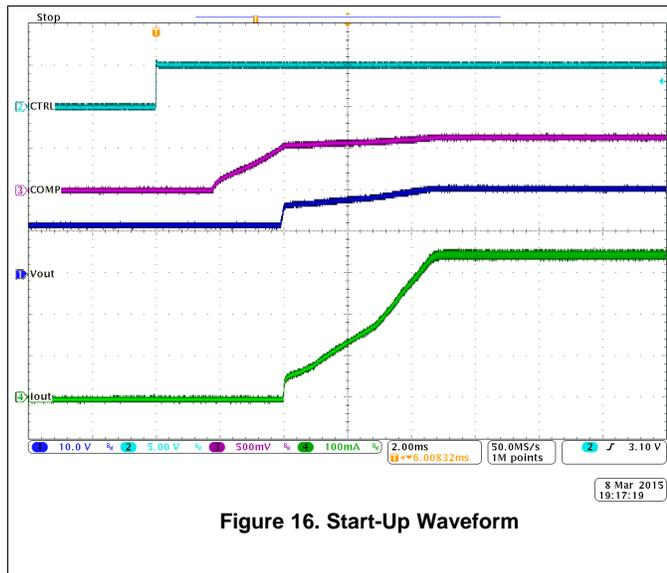
Figure 16. Start-Up Waveform
