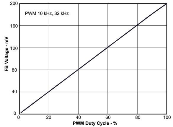
Figure 6. FB Voltage vs PWM Duty Cycle
