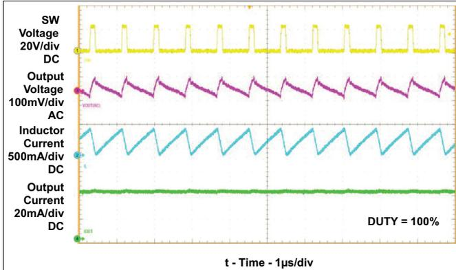
Figure 21. Switching Waveform
