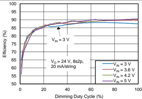
Figure 19. Efficiency vs Dimming Duty Cycle
