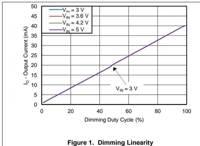
Figure 1. Dimming Linearity
