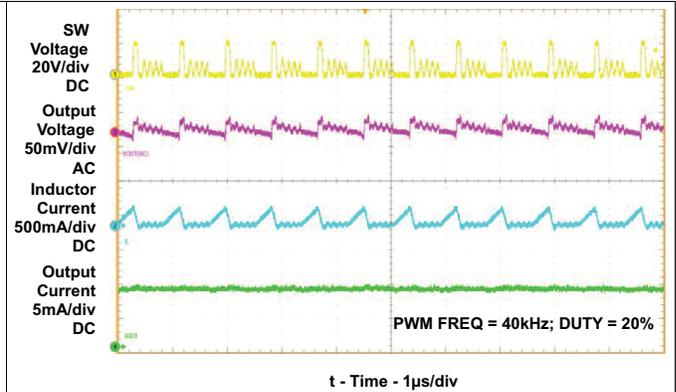
Figure 22. Switching Waveform
