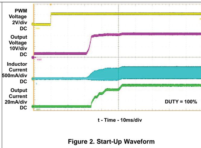
Figure 2. Start-Up Waveform
