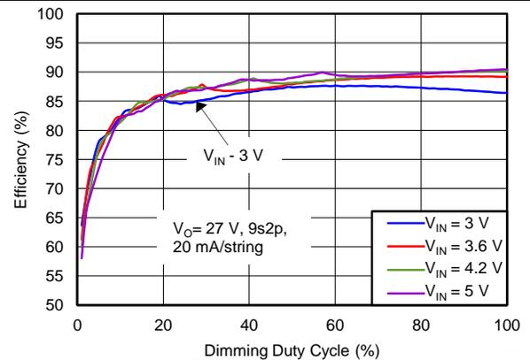
Figure 20. Efficiency vs Dimming Duty Cycle
