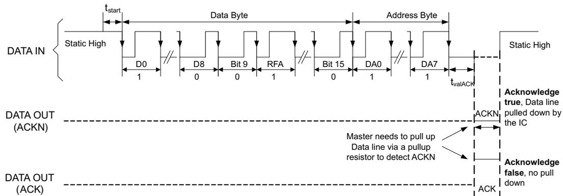
**Figure 12. Easyscale Timing With RFA = 1**
