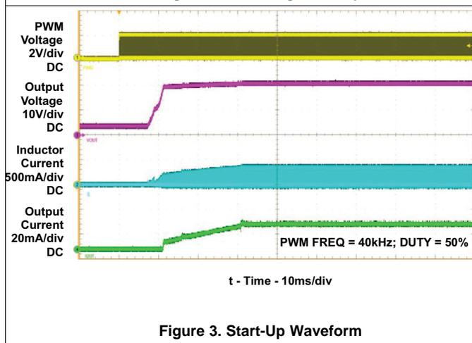
Figure 3. Start-Up Waveform
