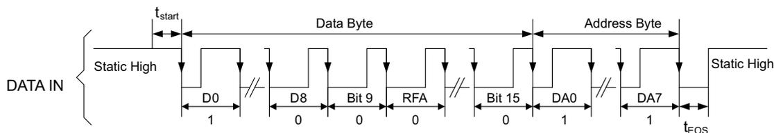
Figure 11. Easyscale Timing With RFA = 0
