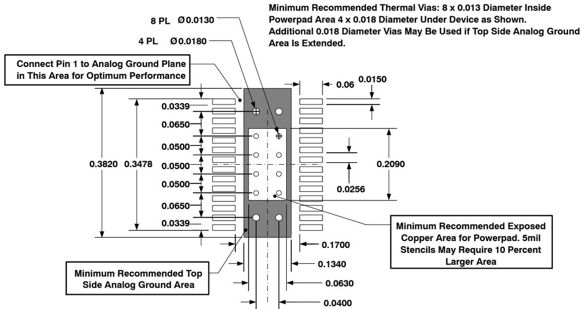
Figure 10. Recommended Land Pattern for 28-Pin PWP PowerPAD
