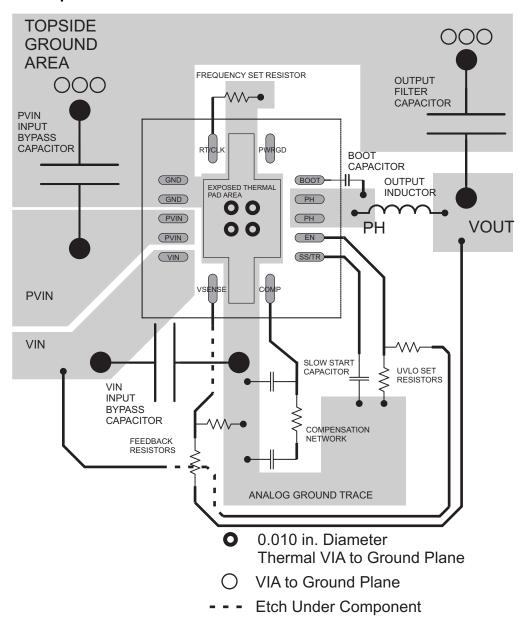
Figure 48. PCB Layout
