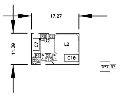
Figure 49. Ultra-Small PCB Layout Using TPS54623 (PMP4854-2)
