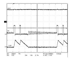
Figure 28. TPS54623 Operation In Pulse Skipping Mode
