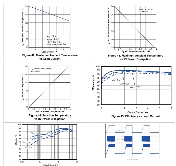
Figure 46. Efficiency vs Output Current
