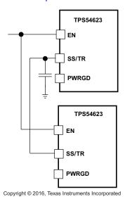
Figure 21. Ratiometric Start-Up Sequence
