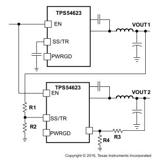
Figure 22. Ratiometric and Simultaneous Start-up Sequence
