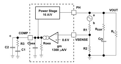
Figure 23. Small Signal Model for Loop Response
