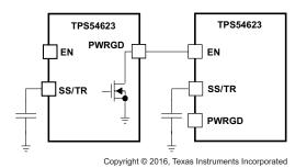
Figure 20. Sequential Start-Up Sequence
