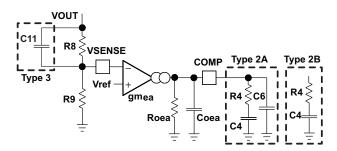
Figure 26. Types of Frequency Compensation
