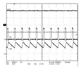
Figure 27. TPS54623 Operation In Current Mode
