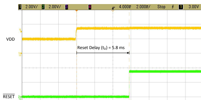
Figure 55. TPS3840EVM \overline{\text{RESET}} Time Delay ( t_D ) with 0.01- \mu F Capacitor
