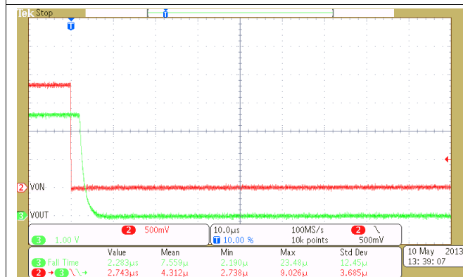
Figure 23. Turnoff Response ( C_{IN} = 1 \mu F , C_L = 0.1 \mu F , R_L = 10 \Omega , V_{IN} = 3.6 V , T_A = 25^\circ C )
