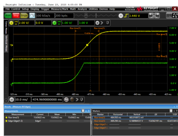
Figure 6. Power Up, 15 ms, V_{BIAS} = 6.5\text{ V} , R_{BIAS} = 0.5\text{ k}\Omega
