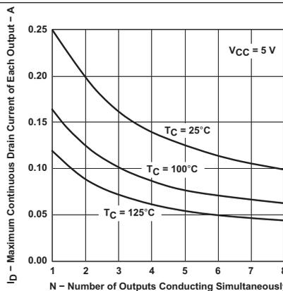
Figure 6. Maximum Continuous Drain Current of Each Output vs Number of Outputs Conducting Simultaneously
