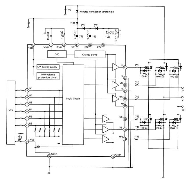
\*1: Optimum conditions depend on the switching loss, EMI, etc., of the external MOSFET.
